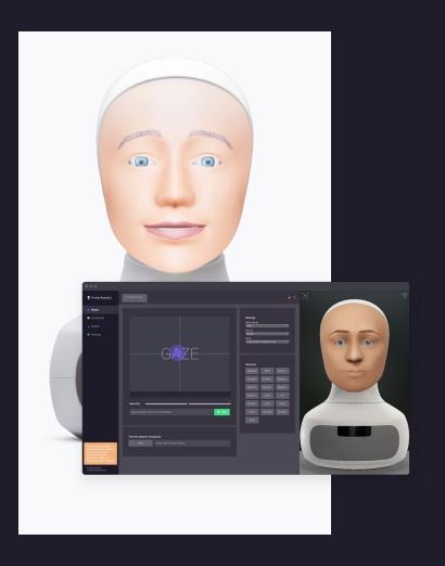
The Virtual Furhat, in its current form, is intended to be used for development purposes for simulating interactions with the Furhat robot.
